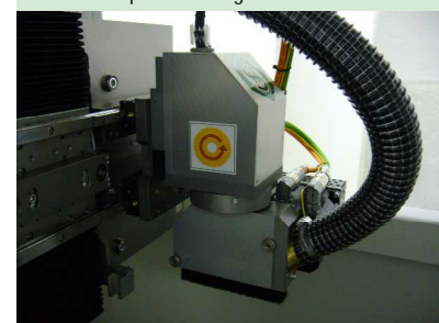
Disc depanelling module with vision system
